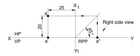
12. (46) A point is lying on HP, 20 mm behind VP and 35 mm behind / infront / from RPP. Draw its projections and name the side view.
