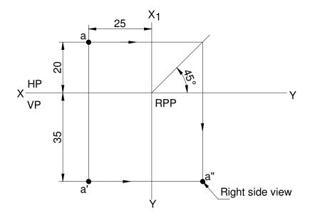
7. (47) A point is 35 mm below HP, 15 mm behind VP and 25 mm behind / infront / from RPP. Draw its projections and name the side view.
