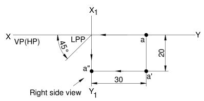
14. (45) A point is lying on VP, 10 mm below HP and 30 mm behind / infront / from LPP. Draw its projections and name the side view.
