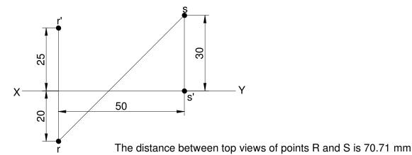
36. (13), (37) A point M is on HP and 30 mm infront of VP. Another point N is 20 mm below HP and 20 mm infront of VP. The distance between their projectors measured parallel to XY line is 50 mm. Find the distance between front views of the point M and N.
