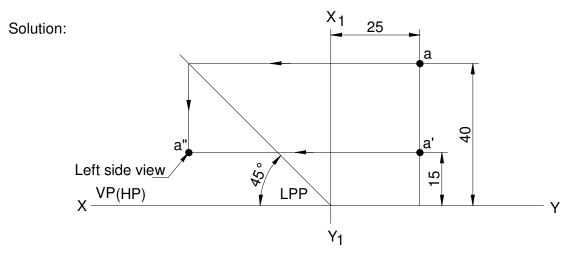
5. (43) A point is 40 mm behind VP, 20 mm above HP and 30 mm infront / Behind / from LPP. Draw its projections and name the side view.
