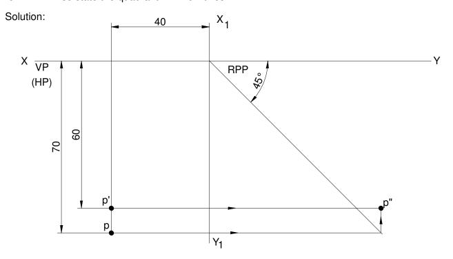
9. (20) A point is 30 mm behind VP, 30 mm above HP and 25 mm infront / behind / from LPP. Draw its projections and name the side view.
