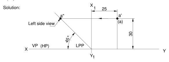
10. (44) A point is 30 mm behind VP, 30 mm above HP and 20 mm infront / behind / from RPP. Draw its projections and name the side view.
