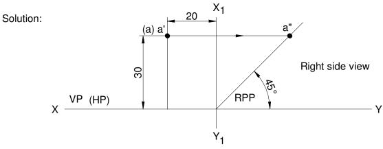
11. (21) A point is lying on HP, 20 mm behind VP and 25 mm behind / infront / from RPP. Draw its projections and name the side view.
