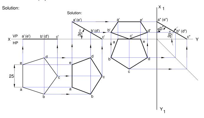
39. (28) A regular pentagonal lamina of 25 mm side is resting on one of its sides on HP while the corner opposite to this side touches VP. If the lamina makes an angle of 60 deg. with HP and 30 deg. with VP. Draw the projections of the lamina.
