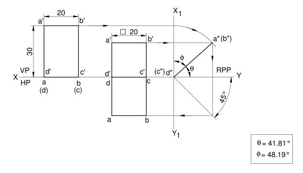
33. (11) The top view of a square lamina of side 30 mm is a rectangle of sides 30 mm X 20 mm with a longer side of the rectangle being parallel to both HP and VP. Draw the top and front views of the square lamina. What is the inclination of the lamina with HP and VP.
