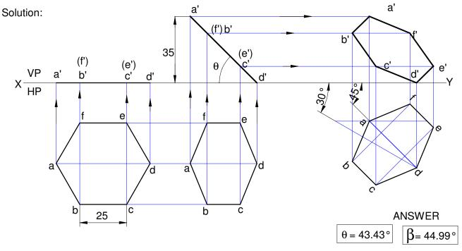
28. (44) A hexagonal lamina of sides 25 mm rests on one of its sides on VP. The side opposite to the side on which it rests is 30 mm infront of VP and the side on which it rests makes 45 deg. to HP. Draw its projections. Also determine the inclination of the lamina with the reference plane.
