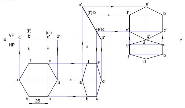
43. (33) Draw the top and front views of a hexagonal lamina of 30 mm sides having two of its edges parallel to both HP and VP and one of its edges 10 mm from each of the planes of projection. The surface of the lamina is inclined at an angle of 60 deg. to the HP.
