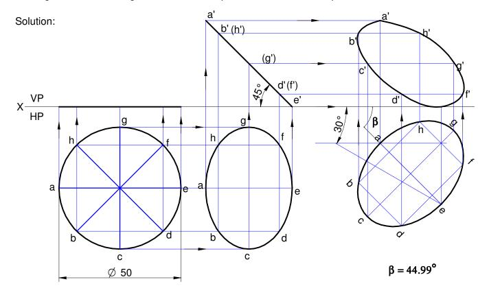
15. (50) A circular lamina of 30 mm diameter rests on VP such that one of its diameter is inclined at 30 deg. to VP and 45 deg. to HP. Draw its top and front views in this position.
