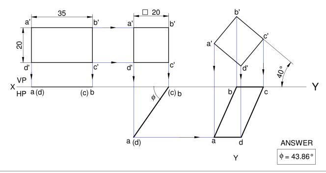
32. (16) The front view of a rectangular lamina of sides 30 mm X 20 mm is a square if 20 mm sides. Draw the projections and determine the inclination of the surface of the lamina with HP and VP.
