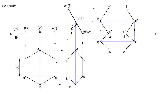
41. (37) A regular hexagonal lamina of side 25 mm is lying in such a way that one of its corners on HP while the corner opposite to the corner on which it rests on VP. If the lamina makes 60 deg. to HP. Draw the projections of the lamina.
