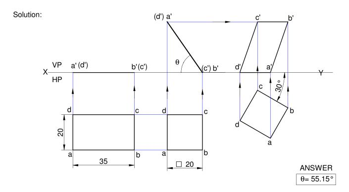
30. (13) A rectangular lamina of 35 X 20 mm rests on HP on one of its shorter edges. The lamina is rotated about the edge on which it rests till it appears as a square in the top view. The edge on which the lamina rests being parallel to both HP and VP. Draw its projections and find its inclinations to HP and VP.
