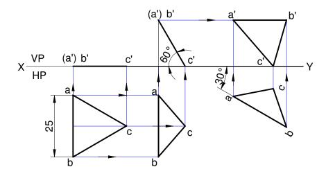
3. (6) A 30 - 60 deg. set square of 60 mm longest side is so kept such that the longest side is in HP making an angle of 30 deg. with VP. The set square itself is inclined at 45 deg. to HP. Draw the projections of the set square.
