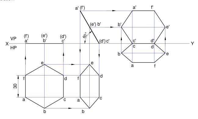
41. (36) A regular hexagonal lamina of sides 25 mm is lying in such a way that one of its sides on HP while the side opposite to the side on which it rests on VP. If the lamina makes 60 deg. to HP. Draw the projections of the lamina.
