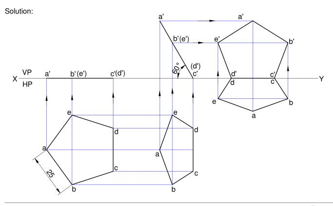
38. (26) A regular pentagonal lamina of 25 mm side is resting on one of its corner on HP while the side opposite to this corner touches VP. If the lamina makes an angle of 30 deg. with HP and 60 deg. with VP. Draw the projections of the lamina.
