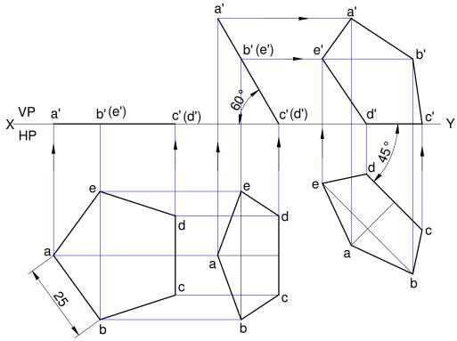
7. (20) Pentagonal lamina of edges 25 mm is resting on HP with one of its corners such that the plane surface makes an angle of 60 deg. with HP. The two of the edges containing the corner on which the lamina rests make equal inclinations with HP. When the edge opposite to the corner makes an angle of 45 deg. with VP and nearer to the observer. Draw the top and front views of the plane lamina in this position.
