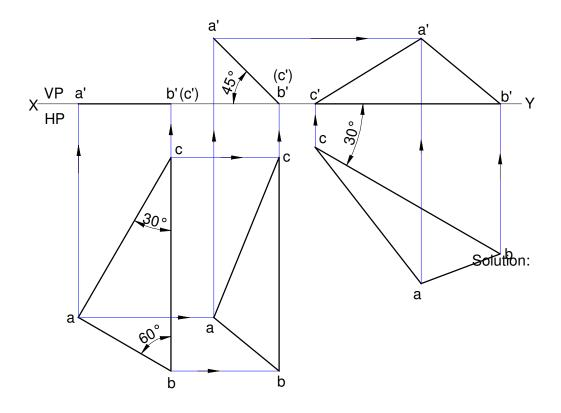
4. (8) A square lamina of 40 mm side rests on one of its sides on HP. The lamina makes 30 deg. to HP and the side on which it rests makes 45 deg. to VP. Draw its projections.
