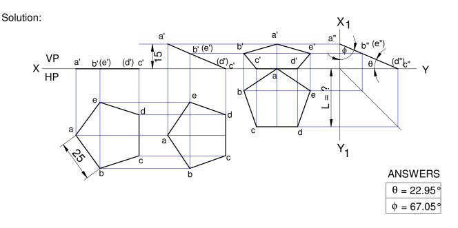
35 (24) A pentagonal lamina of sides 25 mm is having a side both on HP and VP. The corner opposite to the side on which it rests is 15 mm above HP. Draw the top and front views of the lamina.
