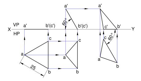
2 (4) A Triangular plane figure of sides 25 mm is resting on HP with one of its corners, such that the surface of the lamina makes an angle of 60 deg. with HP. If the side opposite to the corner on which the lamina rests makes an angle of 30 deg. with VP. Draw the top and front views in this position.
